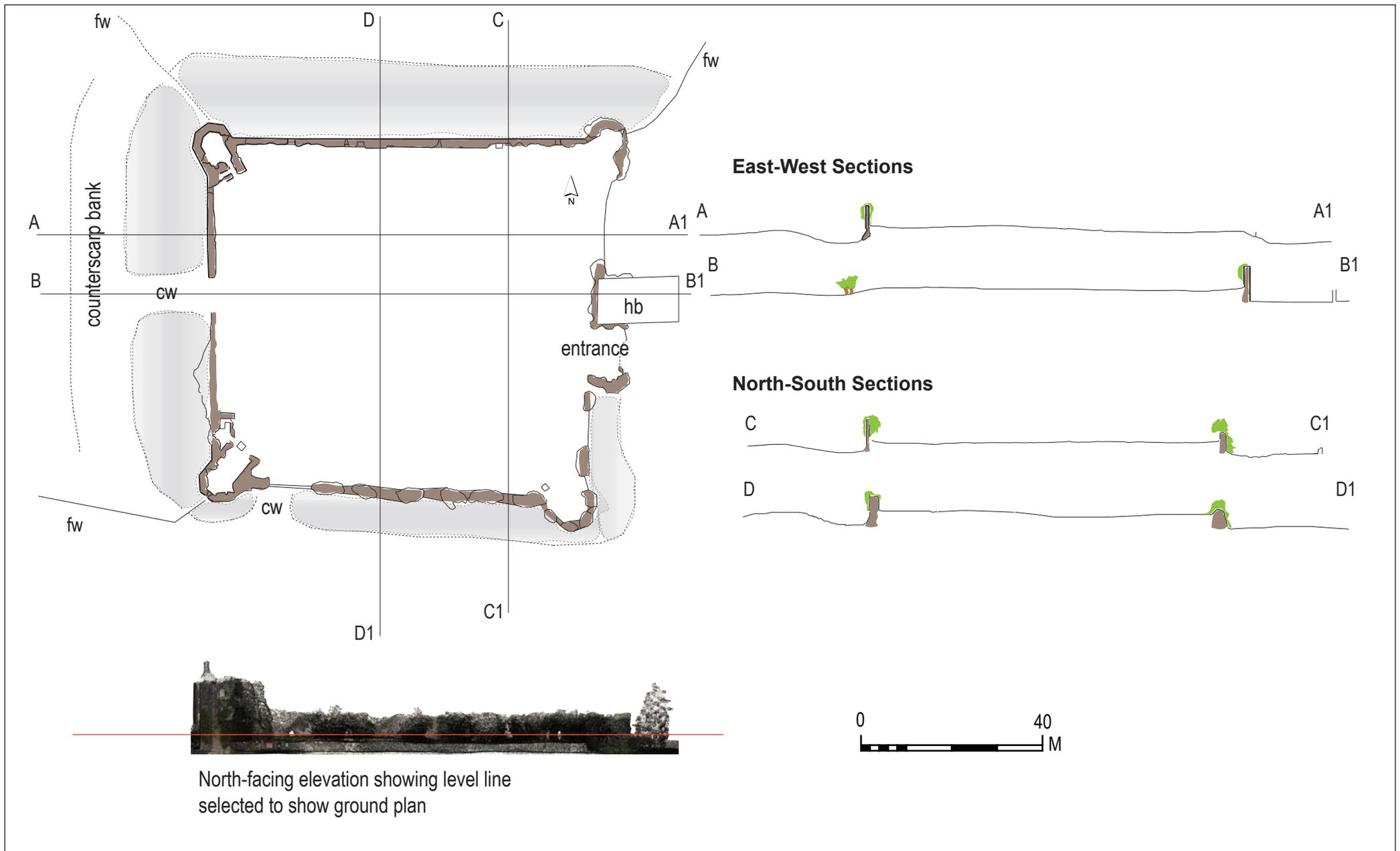
Figure 14: Ballintober Castle, ground plan and sections, 2014
